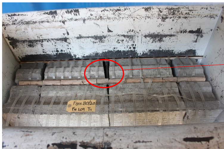
Figure 2: Visual test results sample of inside the VFC block system after completion
