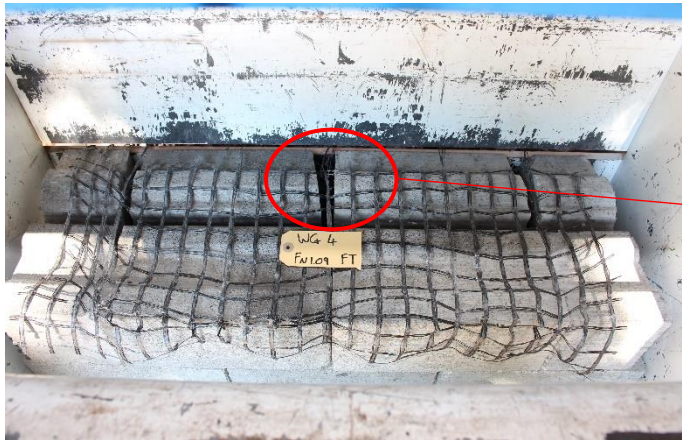
Figure 2: Visual test results sample of inside the VFC block system after completion
