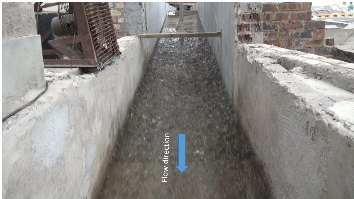
Figure 3-3: Photograph of the flow patterns at the maximum discharge of about 160 L/s when failure is imminent for the 1:10 slope
