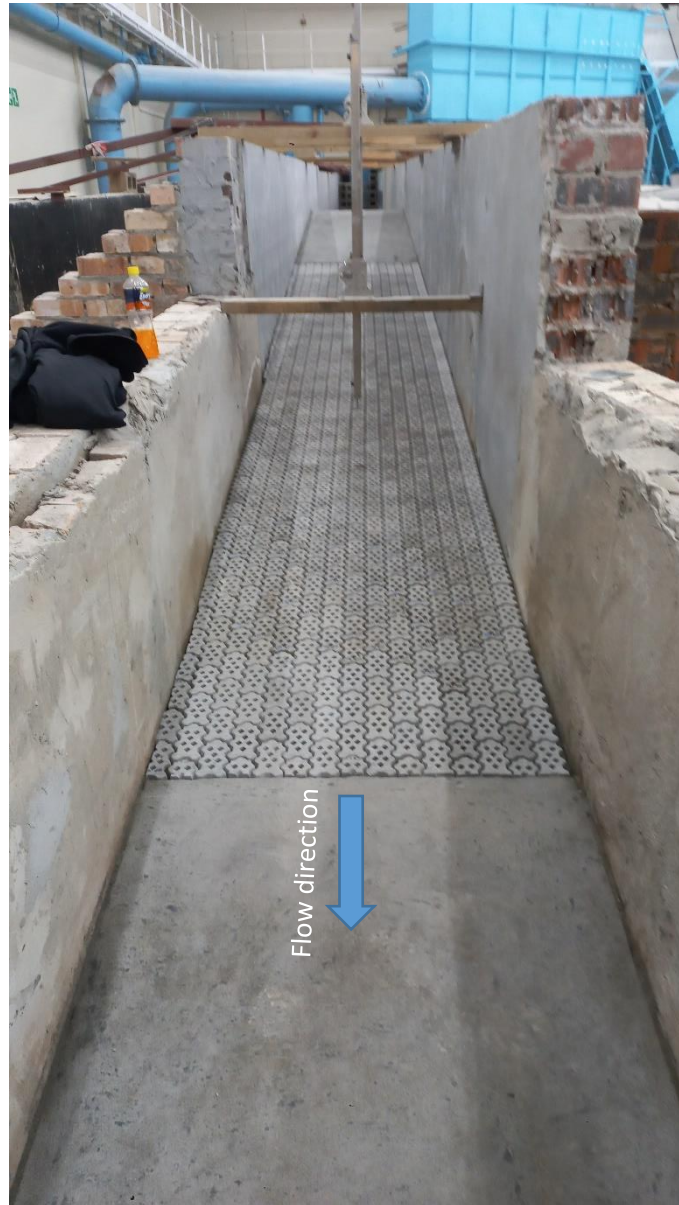
Figure 3-2: Photograph showing the Bosun Buffalo blocks installed in the physical model for the most stable orientation (noses pointing upstream) on the bed slope of 1:10 (V:H)
